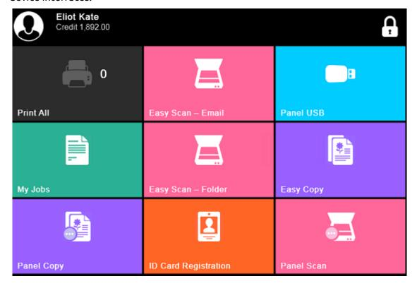
The Embedded Lite terminal, for low-end Kyocera devices, provides the option of secured print without the need of further installation of any software into the device.
