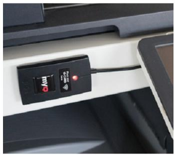
You can also attach it to the printing device or to the MyQ Touch Panel using the TRH holder. The design of the TRH holder provides the possibility to utilize some of the existing holes of the printing device.
