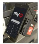
A card reader is connected to the terminal via a USB cable and it is automatically detected after plugged in.
