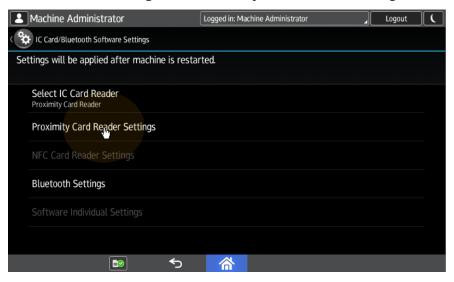
11. Plug in the card Reader to the Android panel via Mini USB — USB (female) reduction. The Proximity Card Reader Settings message box informs you that a USB card reader was registered.
