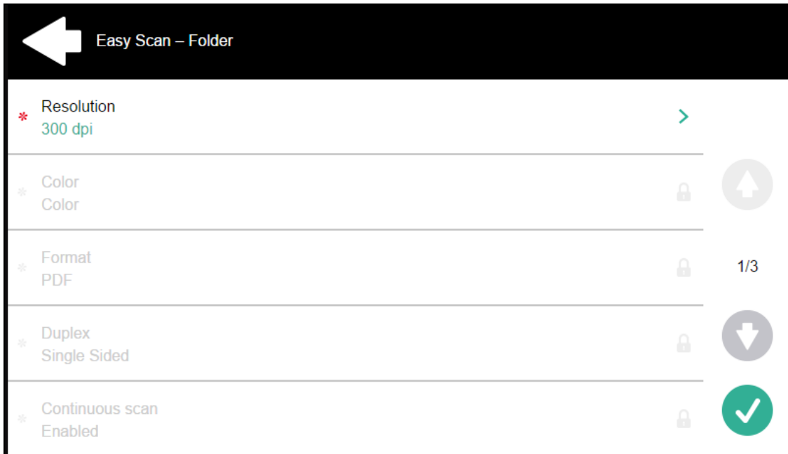
FIGURE 7.92. The Resolution setting can be changed on the terminal screen, other settings are locked.
