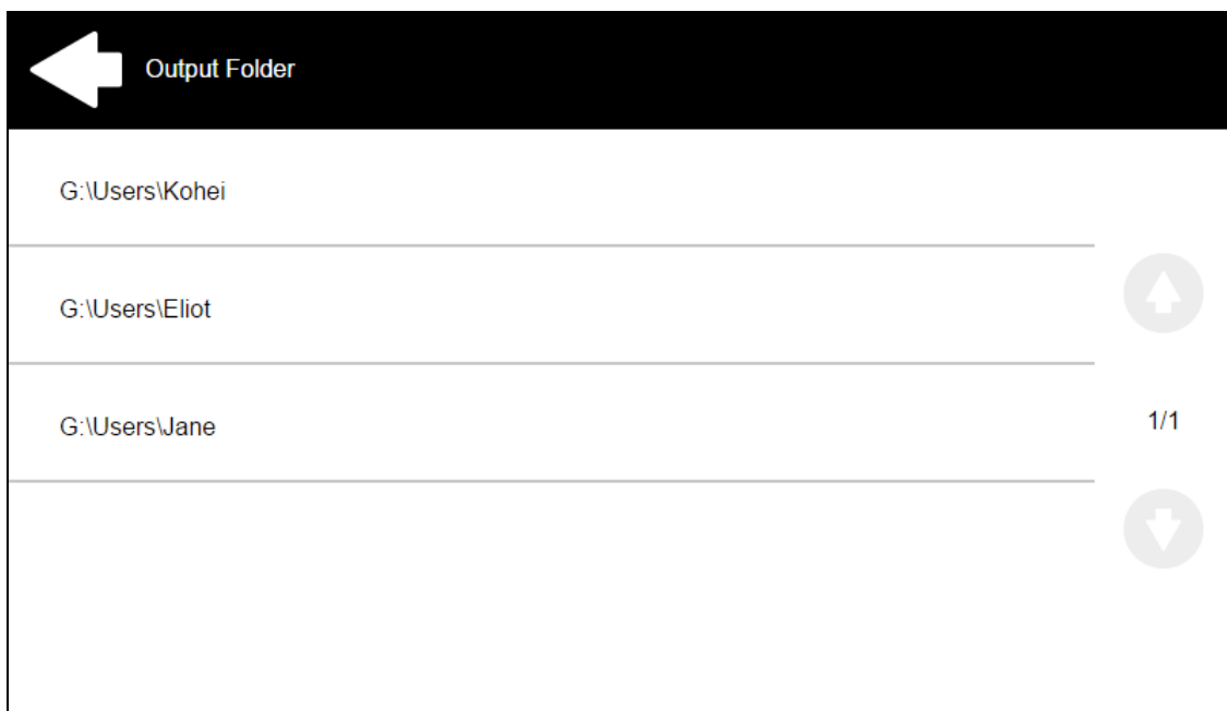
FIGURE 7.113. Users can select the destination on the Output folder screen of the embedded terminal
