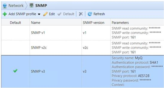
Only use SNMPv3 with a strong password and configure more secure cryptographic algorithms to be used (SHA1 and AES):
